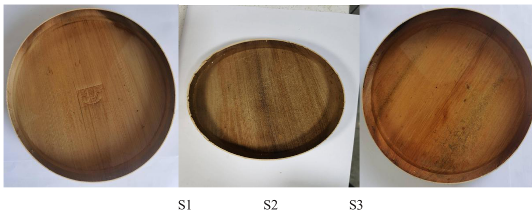
Figure 5. Water leakage of three container groups after 2 h
